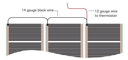
Now go back to the film panel you started with and connect the right corners in the same way with white wire. At the last corner connect a piece of 12 gauge wire that is long enough to easily reach the junction box or thermostat.
