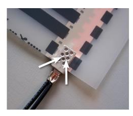
Place the connector over the copper strip on a corner of the film and crimp it so that the teeth on the connector bite into the copper strip.
