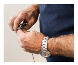
Strip the insulation from one end of a 3-foot length of 14 gauge stranded black wire. The wire is double insulated be sure to strip both layers of insulation.
