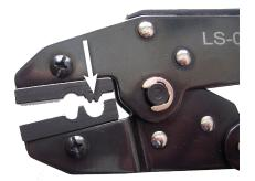
Use only the crimping tool designed specifically for this type of connector. Using any other type of tool could result in loose connections.
