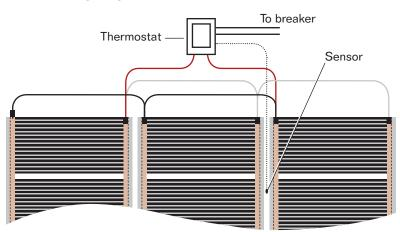
Note that the film panels are wired in parallel.
