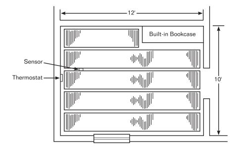
Because of the layout of the room in this drawing, the film panels are about 1 inch apart and about 2 inches from the walls. Your panels may be closer or farther apart but should never overlap.
