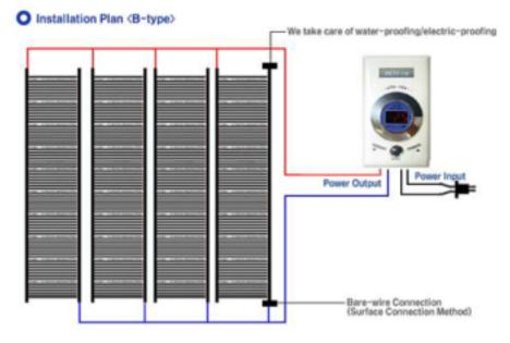
9. The cold ends can be laid in grooves cut in to the insulation for convenience and ease of fitting, the cold ends should not cross under or over the heating film. It is advisable to label and identify the individual cold tails to the heating film for ease of wiring (the heating film do not have a polarity).
