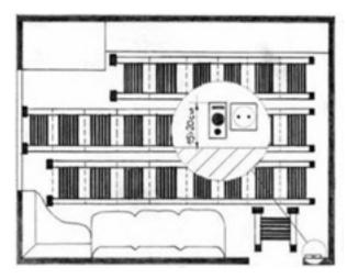
Leave a space and padding around the perimeter of the room size from 4"-8"(10 to 20 cm) spacing between the strips of film - not more than 2"(5 cm) and no less than 1/2"(1 cm)
